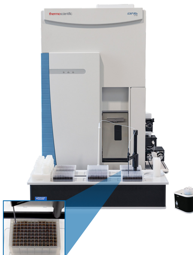
Figure 3. SampleSense FAST UHT-C 4DX and pergo 2 on the Thermo iCAP RQ ICPMS with six microplates. Closeup image shows diluted blood being sampled from microplate well.
